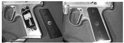
Remove the 2 screws that hold left side panel in place. Connect the battery to the terminal and place the battery inside the grip frame carefully, being sure that the black and red wires to the terminal are not stressed. Make sure that there are no abrupt kinks and the wires are comfortably placed, do not force them into place. Replace the side panel and 2 screws.
