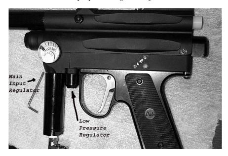
The *BKO* operates on a proven and innovative system. Take the time to understand this section. The pressurized gas is regulated internally. The pressure regulator is
