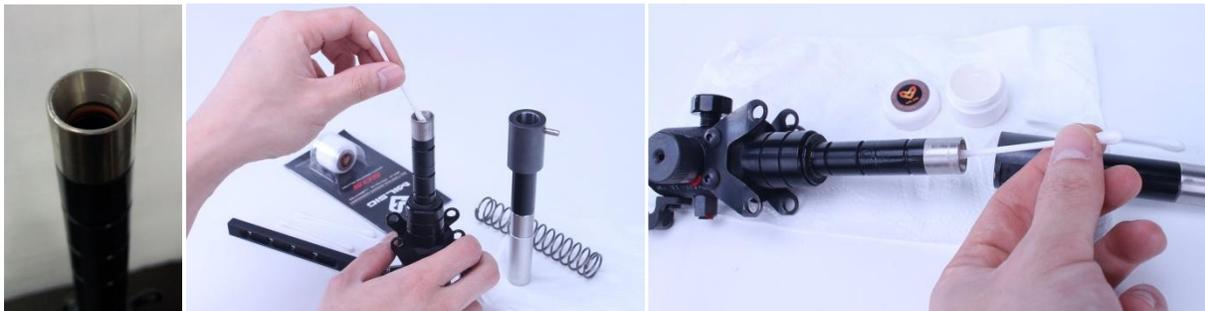
Carefully clean this o-ring with Q-tip and re-oil with SOS lube. *This is the most important maintenance step. This o-ring is made from special material for the most critical and demanding seal in the system. Do not use anything other than well mixed SOS lubricant. (Viton® Fluoroelastomer O-Rings Resists chemicals and oil.)*
