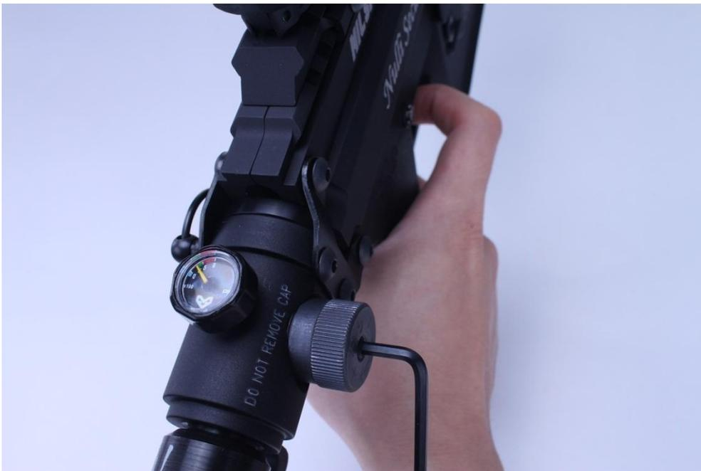
Figure 13 Fire two shots to allow the pressure inside the marker to stabilize before chronoing.
