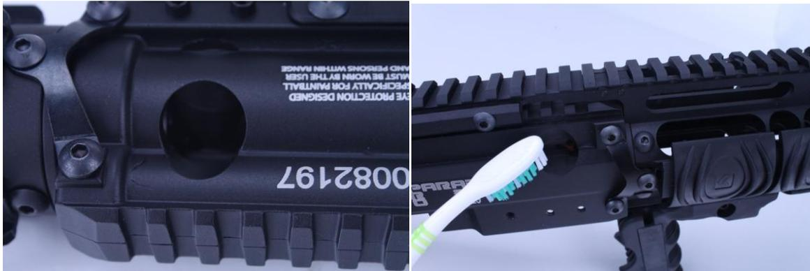
Run a squeegee through the marker barrel with warm soapy water until paint and or damage debris are removed. Use a tooth brush for stubborn paint. Then wipe dry with paper towel and blow dry.
