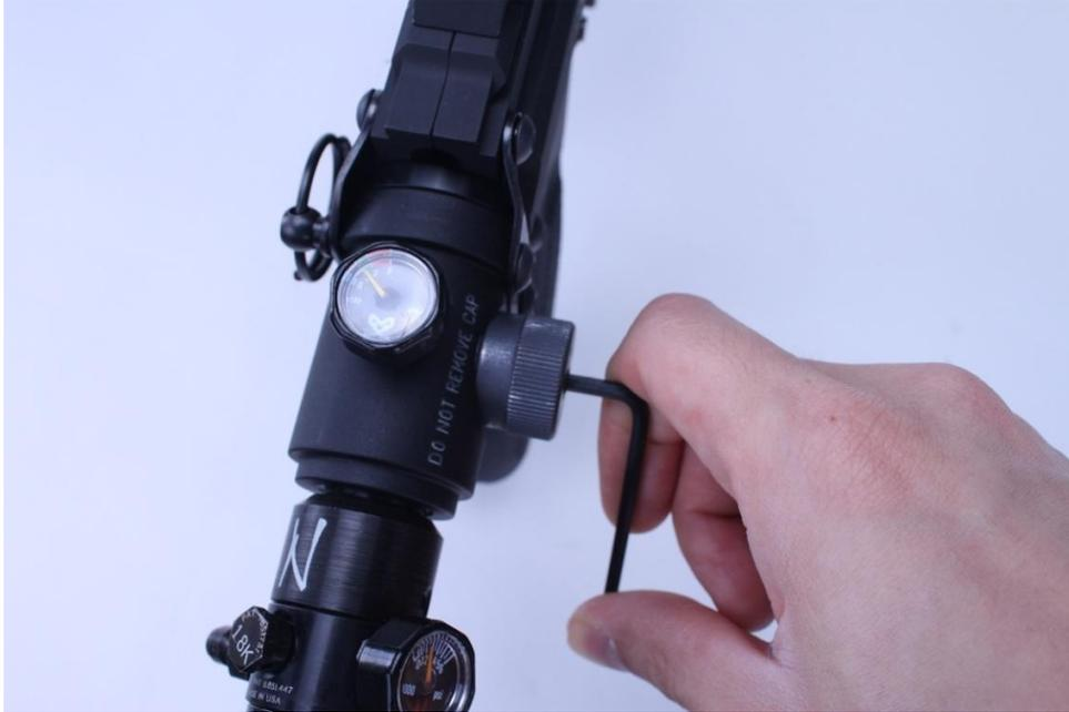
Figure 14 Dial down the fps to your field's limit. Fire twice to allow marker's pressure to stabilize.
