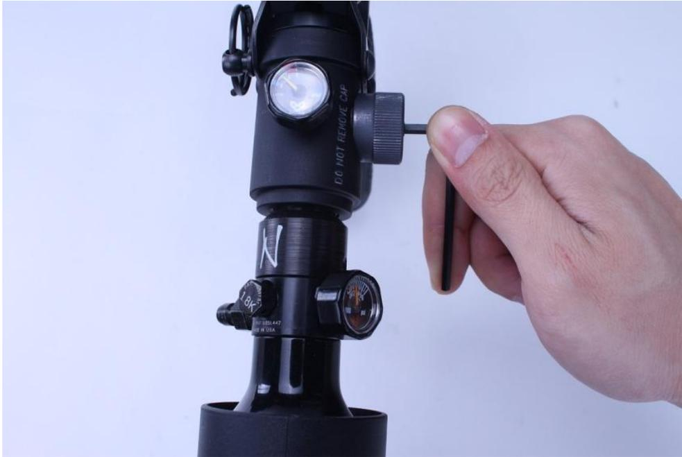
Figure 12 Open up the regulator to increase marker's pressure until indicator reach green zone.
