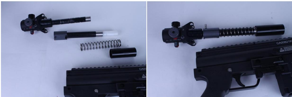
Insert the HEAR Core back into the marker sideways.
