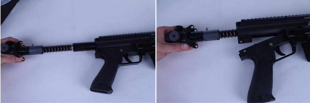
Take care to orientate the hammer guide pin to the top of the receiver body as shown above.
