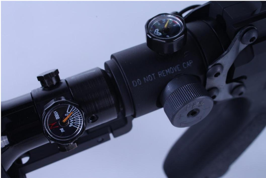
Figure 15 Marker's pressure-gauge indicates the marker's pressure is below green zone. Chances of burping increases.
