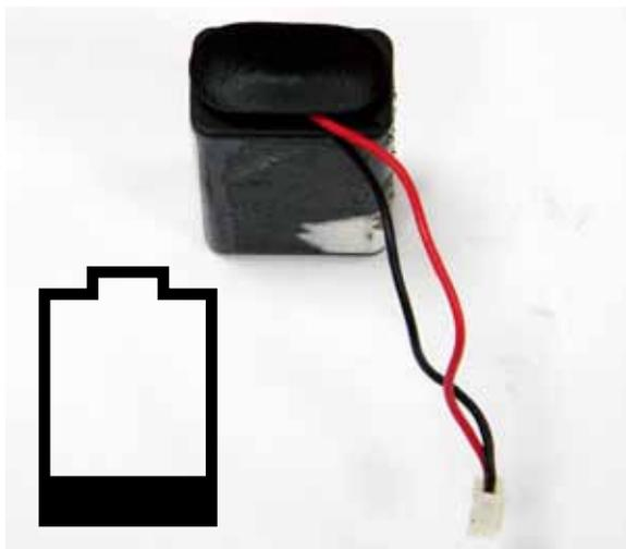
**POSSIBLE CAUSE:** Battery has insufficient power.
