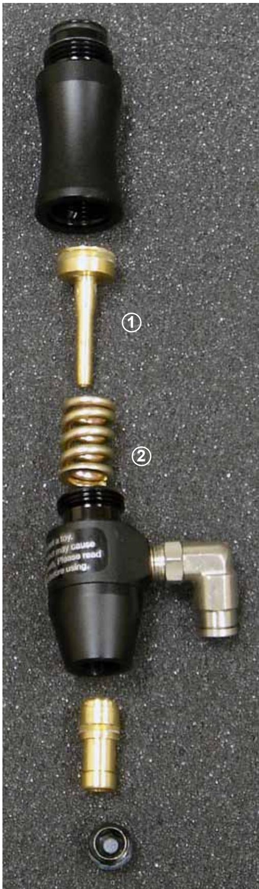
**POSSIBLE CAUSE:** Poorly maintained Inline Regulator.
