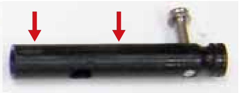
**SOLUTION:** Needs lubrication on striker and bolt.
