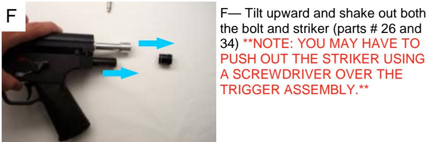
F— Tilt upward and shake out both the bolt and striker (parts # 26 and 34) **\*\*NOTE: YOU MAY HAVE TO PUSH OUT THE STRIKER USING A SCREWDRIVER OVER THE TRIGGER ASSEMBLY.\*\***
