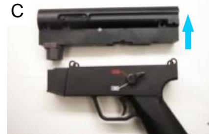
C— Once the Main Body (part # 14) and the Trigger Assembly (part # 39) are apart from one another it will look as picture C. **\*\*NOTE THE SCREW PLACEMENTS.\*\***
