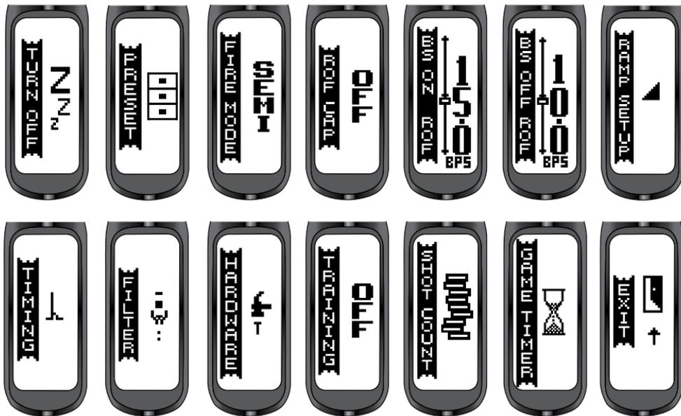
The Main menu contains both editable parameters and sub-menus which contain editable parameters. Some of these parameters affect the way the GEO3.1 shoots and are tournament locked as standard from the factory.<sup>1</sup>
