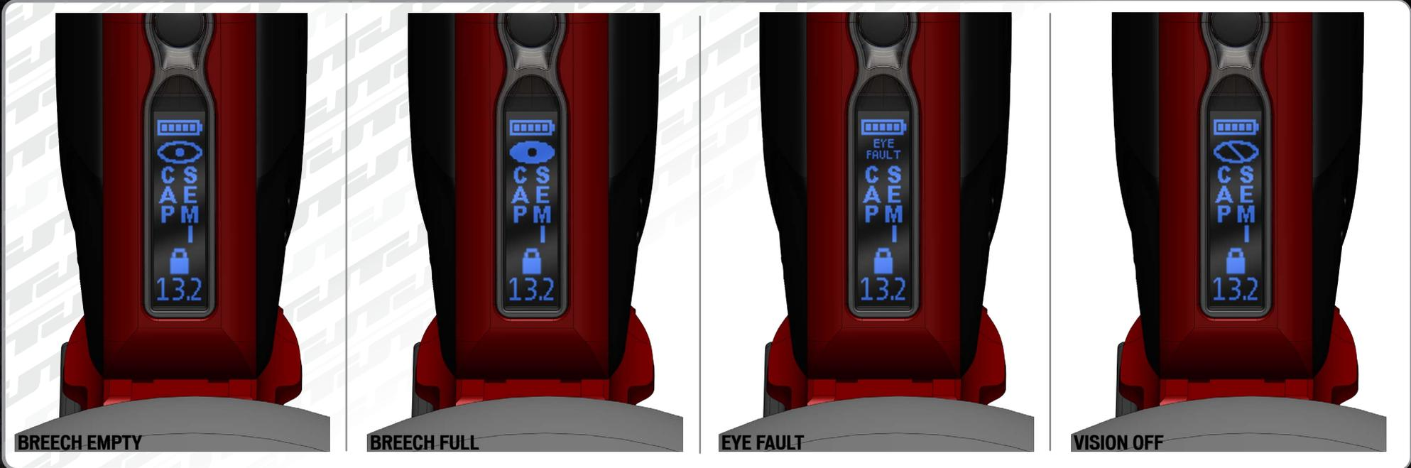
**VISION** The Impulse is equipped with the latest generation Vision™ break-beam anti-chop eye system. Multiple Vision modes may be selected (see programming) and the Vision™ status can be read from the display screen.
