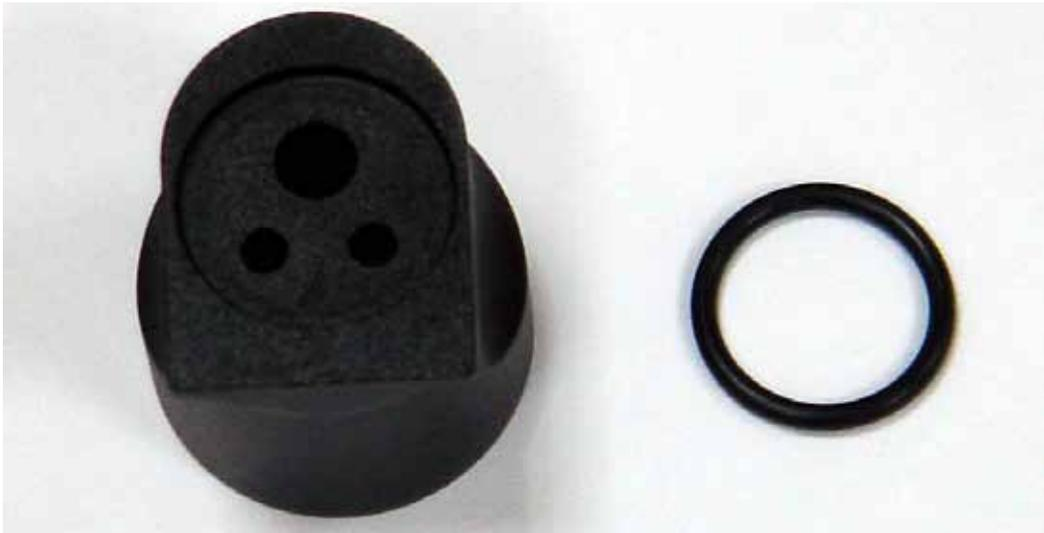
**POSSIBLE CAUSE:** Regulator Seal O-Ring is damaged.
