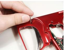
Use an small allen key or skinny pair of needle nose pliers to hold threaded trigger spacer and tighten the attachment screw with 3/32 allen key
