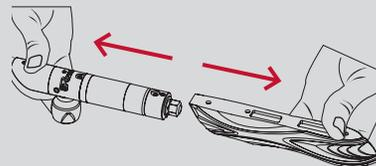
Keeping the body upside down, slide the inner receiver components out of the body cover.
