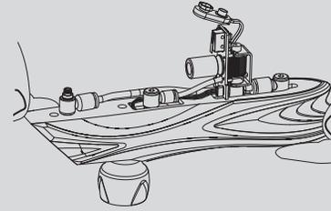
Gently complete the process of separating the body from the grip frame. Take care to make sure that the circuit board slides out of the grip frame without being strained, and that the battery wires and battery clip follow without catching on the grip frame. Set the grip frame aside, and hold the body upside down (with the feedneck facing down.)
