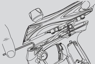
Remove the front banjo fitting from over the vertical adapter with a 1/8-inch allen wrench. The center of the banjo fitting will turn with the wrench, pivoting inside the rest of the fitting.
