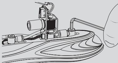
Remove the remaining two banjo fittings from the body with a 1/8-inch allen wrench.
