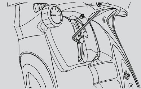
FIG. 15 → ADJUSTING ACTIVATION POINT
