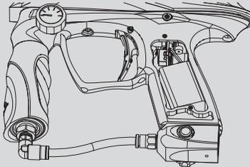
Using a 5/64-inch Allen wrench, remove the two screws from the left side of the rubber grip and lift the panel open. Attach a fresh 9-volt alkaline battery to the battery clip. Position the battery in the grip frame, tucking the battery wires into the space above the battery. Close the grip and reinstall the screws.
