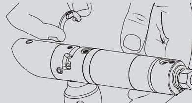
Remove the Vision circuit board from the body breach and set aside carefully. This circuit board is shaped like the letter C, and should come easily out of place. Take care to make sure that the infra-red emitter and detector (these look like clear LEDs) are not set on anything that can scratch them.
