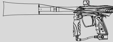
Screw the included barrel into the Epiphany. Put the supplied barrel blocker over the end of the barrel, securing its cord as far back on the Epiphany body as possible, and cinching it tight.
