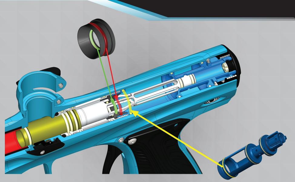
THIS DIAGRAM ILLUSTRATES THE O-RINGS RESPONSIBLE FOR AIR LEAKING FROM INSIDE THE FACE OF THE BOLT.
