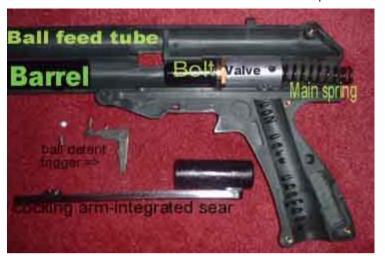
**Cutaway of the NSG Splatmaster**
