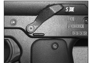
The TM-7 will now be ON and in the Safety Position. To make the TM-7 Live, move the Selector Switch to the desired Firing Mode.
