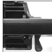
**Note:** Notice how the stock lock sits in the shell before removing it, so it's easier to reinstall.
