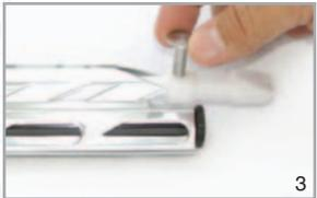
Lift Bolt Pin and Remove Bolt
