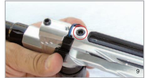
Remove Ram Sleeve Retaining Allen
