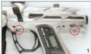
Trigger Assembly Screws
