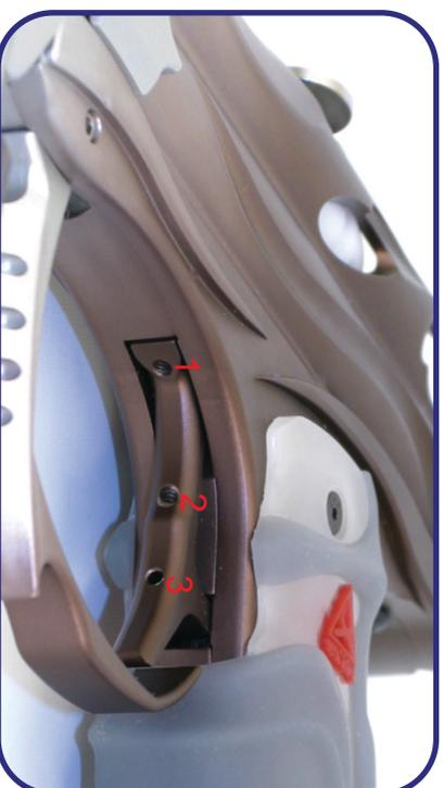
1. Trigger tension. Your NME trigger uses magnetic force to return your trigger. To adjust the force behind the magnet simply turn the .050 allen screw located at the top of the trigger clockwise. To decrease the magnetic force turn the same screw counter clockwise.
