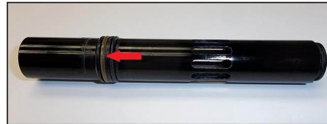
9. Apply grease to the two small O-Rings on the Rod #8a, #8b.
