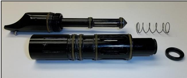
3. Push the Bolt out of the back of the Air Guide.
