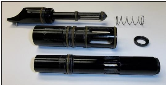
4. Unscrew the Bolt Guide from the Back Cap. Remove old grease and debris from Firing Engine.
