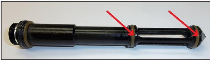
10. Lubricate the 3 inner O-Rings on the Air Guide (#2a, #2b, #2c), no lube is needed on the outer O-Rings.
