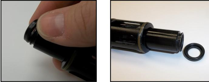
2. Unscrew the Air Guide by turning the Air Guide counter-clockwise to remove from the Back Cap. The Bolt Spring will come out with the Bolt Guide.
