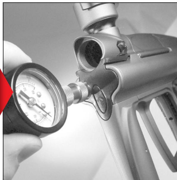
**1** Remove the volume chamber maintenance plug using a 4mm Allen wrench.
