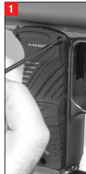
**1** Remove the right hand grip cheek by removing the **3** screws using a suitable 2mm Allen wrench.
