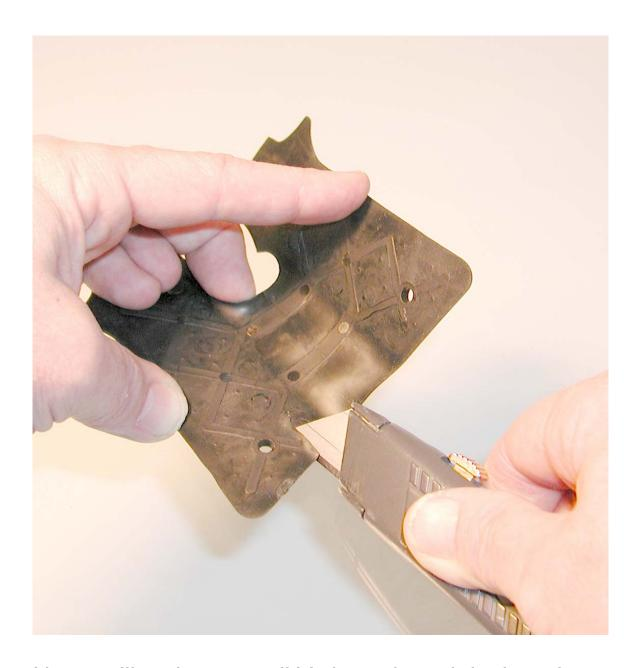
Next we'll make a small V shaped notch in the grip to create a channel for the wire to exit. Careful! Don't cut through the nylon center!
