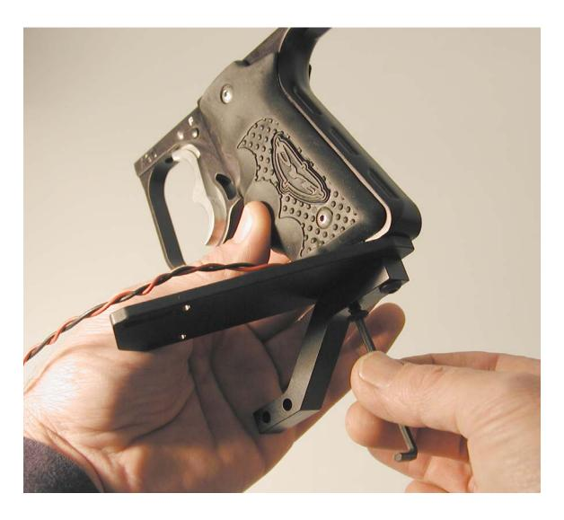
We are setting this marker up for a right handed player and hanging our Warp off the left hand side of the marker. Note the un-slotted end of the Warp Mounting Bracket connects to the grip frame.
