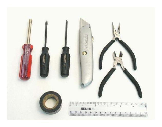
3/32 Nut Driver \* Standard Screw Driver Utility Knife \* Needle Nose Pliers \* Wire Cutters \* Electrical Tape \* Ruler
