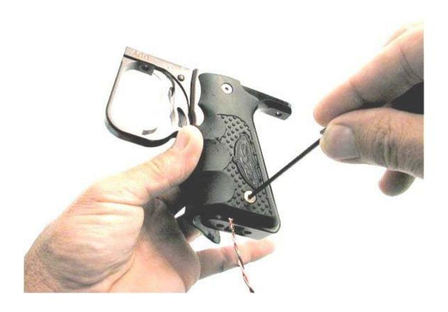
Align the wire with the notch and install the four grip screws.
