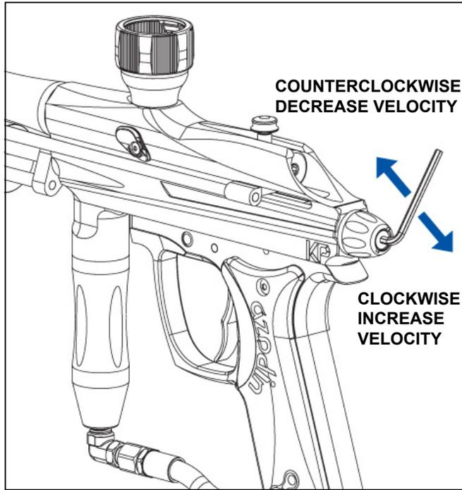
To increase your velocity FPS (Feet Per Second), use the allen wrench to turn the Velocity Adjuster (P023) clockwise.
