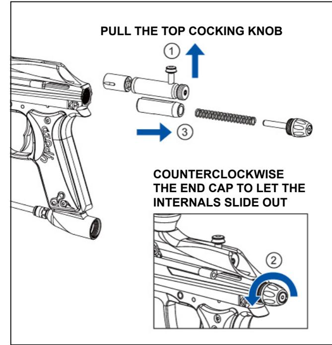
**WARNING:** Never remove the internals of the marker while the air tank is attached with the marker. Always remove all paintballs, loader and air tank before disassembling the marker.
