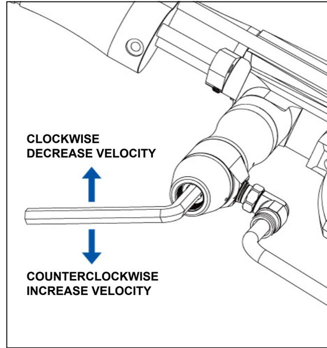
To increase the input pressure use the allen wrench to turn the Regulator Adjustment Screw (S032) counterclockwise.
