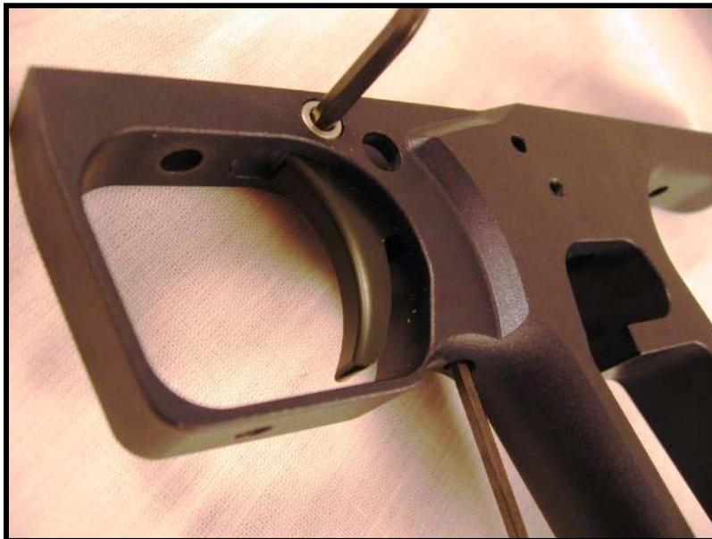
*Above: The access hole to the Undertravel screw is shown by the bottom Allen key.*
