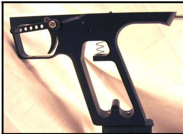
3. Remove the Auto Trigger Arm and Cam from the .45 frame. Sometimes you can simply rotate the AT arm to remove it - if it feels stuck you will most likely have to back out the undertravel screw (see below).
