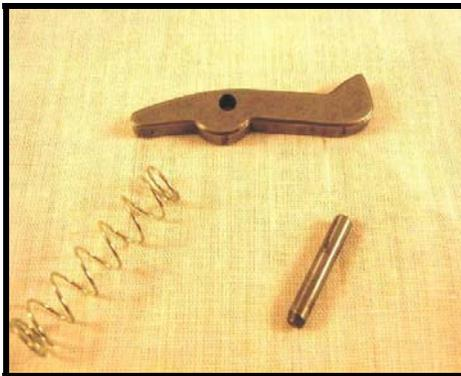
7. Inspect the Sear to see if it has wear where the lug catches. (Notice the slight wear on this sear.) Wear can cause the marker to 'skip' (not recock from time to time) or be VERY hard to time the auto trigger. Replace this if wear is evident or malfunctions are occurring. This should not need to be done often and perhaps will never need to be replaced on your marker.
