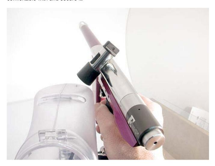
From the side, mark where the center of the feed hose will pass through the hopper.
