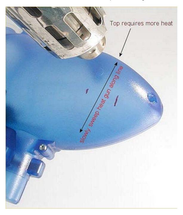
When you see that the plastic is starting to sag, it's time to make the depression with a barrel or length of pipe.
