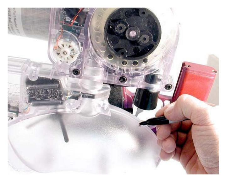
Finally, estimate where the center of the hose will pass through from this angle and mark it.
