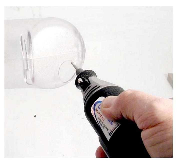
Keep checking your work until the hose will pass through in a direction towards the other hole. A little bit more of this side here and we'll have it!
