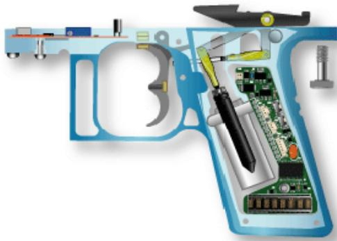
The Grip Frame contains all of the electronics that run the X-mag.
