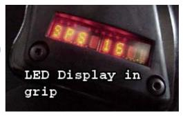
iron core that is linked to the sear. An LED (not LCD) display in the grip frame displays the selected mode, shot counter, game timer, and maximum rate of fire information. Two pushbuttons in the rear of the grip select modes and change settings.
