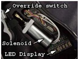
switch in the trigger assembly to be fouled by dust, water or debris. Instead, a sealed hall effect sensor picks up the movement of the magnetic field from another magnet in the trigger, and send a signal to microprocessor in the grip frame.
