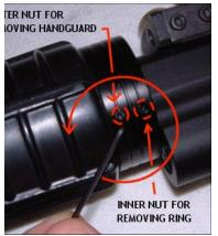
Loosen the lug that holds the sight compression pin, then loosen the the bolt that holds the sling attachment ring Next loosen the lugs on the rear section of the hand guards – the whole assembly should be loose enough to rotate and adjust so its properly aligned for sighting – make sure the barrel is tightly set into the receiver before doing the alignment – then retighten all screws
