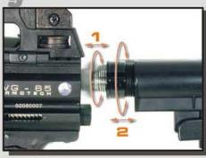
1. Turn Locking Collar Counter Clockwise 2. Turn Entire Rear Stock Unit Counter Clockwise
