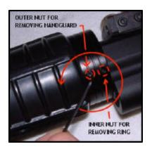
properly aligned in reference to the rear sight (tighten barrel first, align these elements after) in order to have the best performance.
