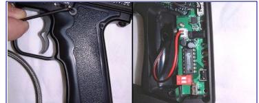
with the pressure gauge) and remove the trigger frame cover.
