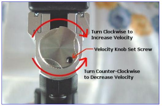
To adjust velocity after loosening the locking retainer screw, turn the velocity screw clockwise in ½ turn increments. To decrease velocities turn the velocity screw counter-clockwise. Once the desired velocity has been reached, lock the velocity screw in place.
