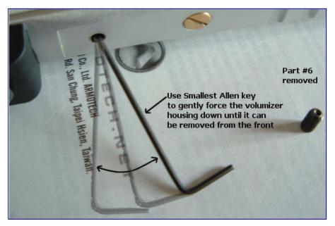
3. Once this part is out, the cupseal, valve stem, spring will all easily be removed for service.
