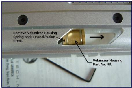
4. When reinstalling please remember to install the valve-stem/cup seal, spring, volumizer housing (copper looking piece) and Co2 cartidge puncture plate in that order. Improper assembly will cause the marker to malfunction.
