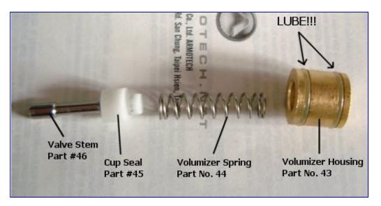
5. Use a flat screwdriver (long stem) to slide the volumizer housing back into place.
