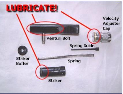
• Lubricate ONLY the sections of the venturi bolt and striker where the o-ring is fitted. These are the only sections which make physical contact with the sidewalls of the receiver internally.
