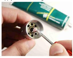
Insert adjustment screw until flush with outside of regulator body.
