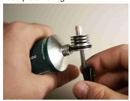
Insert piston with spring pack into center section.
