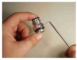
Remove piston from center section with paper mate pen. Using a plastic pen ensures that the piston sealing surface will not be compromised. Place on flat surface and press out.
