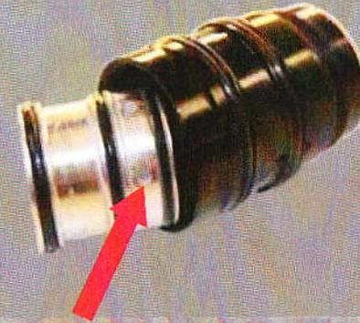
Step #5: Lubricate the bolt o-rings and slide the bolt into the keg.
