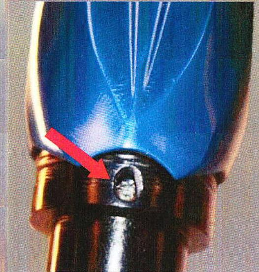
Step #8: If it is slightly misaligned, use a small allen key to place it. Fix the drive train using the top locating screw.
