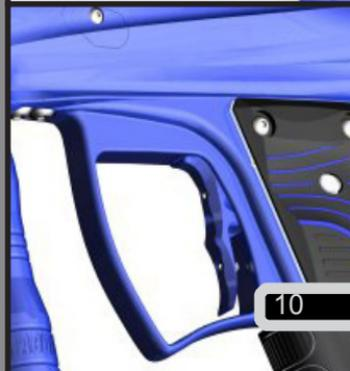
Remove the three screws that hold the wrap around grip on and peel the grip back to allow access to the battery. Remove the old battery, and replace it with a new one. Only use high quality alkaline 9V batteries, the best possible choice is to use a MacDev Militia PowerPack (type 6LR61).
