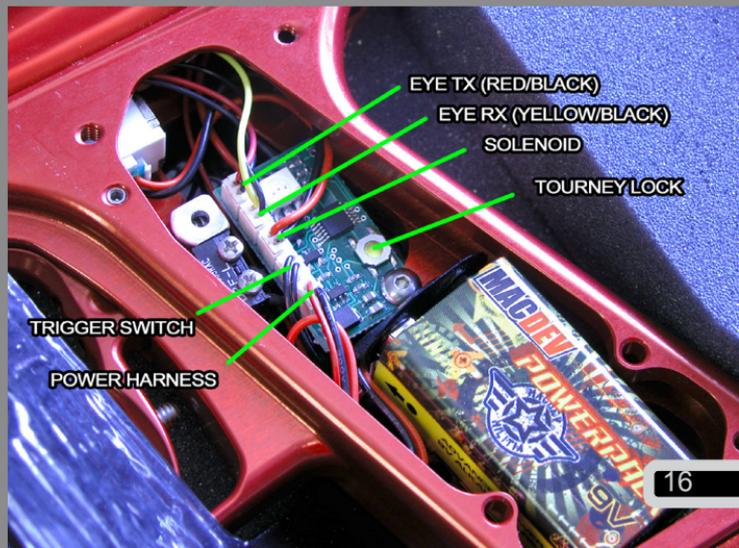
mode (turn the Droid on with the trigger depressed). The indicator LED should now show blue (debounce register). Use a q-tip or similar non metallic, blunt item to depress the tourney lock button as shown. Hold the button for approximately 10 seconds until you see the indicator LED flash a rainbow of colours. The software is now reset to default settings.
