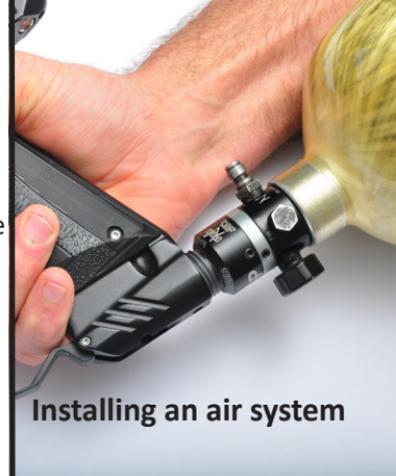
Installing an air system
