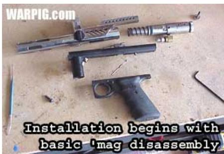
For someone who is familiar with properly maintaining their Automag, armed with the knowledge from Airgun Design's maintenance video, installing the Hyperframe is not a terribly challenging task. It starts with disassembly of the
