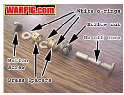
With the valve core removed, a 3/16" allen wrench can be used to remove the hollow nut which holds all of the on/off seals in place. An o-ring pick can be used to remove each of the three white o-rings and two brass spacers which seal the valve. A fourth o-
