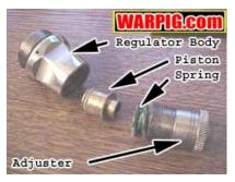
paintgun, the output pressure gauge can further diagnose air venting from the relief valve. If the pressure is normal, it would indicate a damaged relief valve. Unusually high output pressure indicates a dirty or damaged regulator pin.
