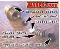
If a bad relief valve seal is indicated, 1/8" allen key is Regulator Piston needed to remove the hollow Relief Seal nut from the top of the Relief Disk regulator piston. Inside is a spring, metal disk, and black poly seal disk. Upon reassembly, the small dimple in the metal disk should be facing the spring.
