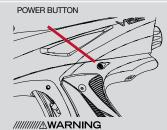
Turn the marker on by pressing the power button, and holding it in for a full second. When the Vibe turns on, the power button will glow red. The Vibe is turned off by pressing and holding the power button for two seconds. To conserve battery power, the Vibe will turn itself off if it is not fired for more than 30 minutes.
