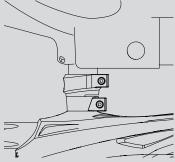
While an un-powered hopper will work, powered loaders will provide better performance, and minimize paint breakage. Snap the Vibe's clamping feedneck over the body's feed port, narrow end facing the marker. Insert the loader's feedneck into the larger end. Align the loader, and tighten both the top and bottom sides of the clamping feedneck with a 7/64-inch allen wrench.
