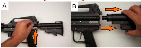
A—Loosen stock retaining screw (part #19) With a 3mm Allen Key B—Remove stock by pulling towards the direction shown.
