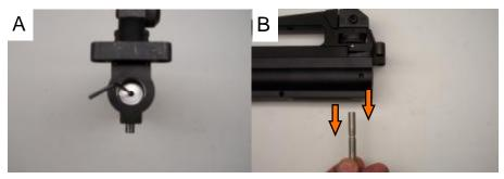
A— Begin by unscrewing the Connector Pin retaining screw (part #18) 3 turns with a 2mm Allen key. \*\*\*NOTE: DO NOT REMOVE THIS SCREW.\*\*\*
