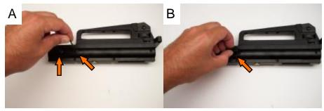
A— Begin by removing the Ball Detent Retaining screws (part # 10 &11) B— Pull out the Ball Detent (part #9) in a upward then out motion as shown in picture 'B'
