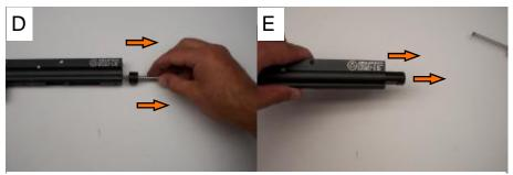
D— Pull out the Velocity Guide pin (part #29), the Velocity spring (part #30), and striker cushion (part #31)
