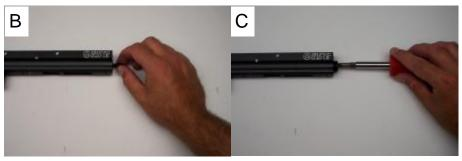
B—Loosen and remove velocity screw (part# 27)
