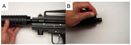
A— Begin by unscrewing the barrel from the top body half in a counter clockwise motion as shown.
