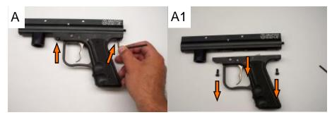
A and A1—Begin by removing the trigger assembly screws (part #55) with a 3mm Allen key on the front and rear of the trigger assembly. The bottom body half and trigger assembly will now come apart as shown on picture A1.
