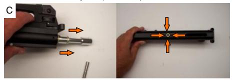
C— Tilt the upper body to slide the bolt (part # 15) towards the back of the marker and remove by pulling towards the direction shown.
