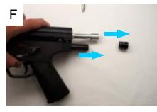
F— Tilt upward and shake out both the bolt and striker (parts # 26 and 34) \*\*NOTE: YOU MAY HAVE TO PUSH OUT THE STRIKER USING A SCREWDRIVER OVER THE TRIGGER ASSEMBLY.\*\*
