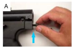
A—Begin by unscrewing the Velocity Adjustor Screw (part # 29)
