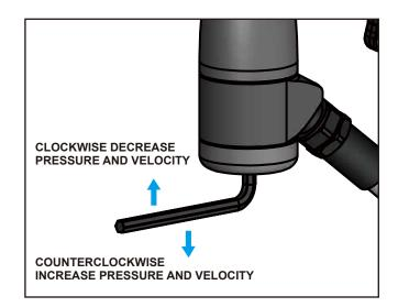
To increase the input pressure, use the allen wrench to turn the Rock Steady Seat (RSS3) counterclockwise.
