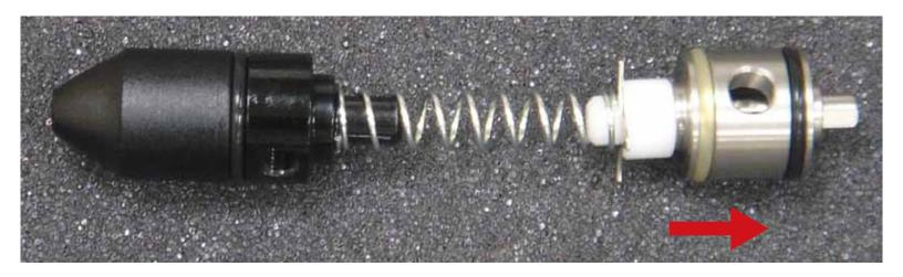
POSSIBLE CAUSE: Cup Seal Guide is jammed in the valve
