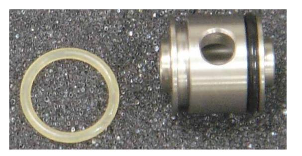
POSSIBLE CAUSE: Front Valve O-Ring (R012) is damaged
