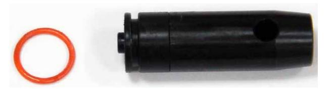
POSSIBLE CAUSE: Striker O-Ring is damaged.
