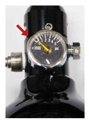
POSSIBLE CAUSE: insufficient air supply ( HPA)
