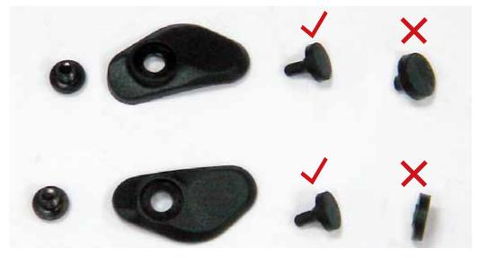
POSSIBLE CAUSE: Ball Detents are damaged
