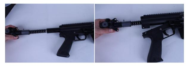
Take care to orientate the hammer guide pin to the top of the receiver body as shown above.
