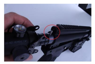
Figure 10 Check the bolt guide is secured and is in the correct orientation before reinserting.
