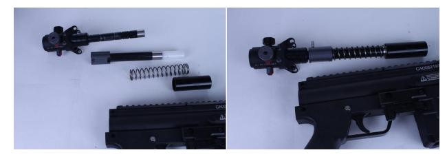
Insert the HEAR Core back into the marker sideway.
