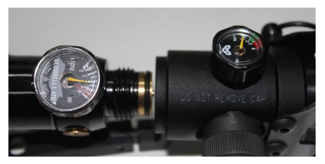
Figure 11 Always insert the 13Cl bottle or Air Source that is pressurized to over 1000psi.
