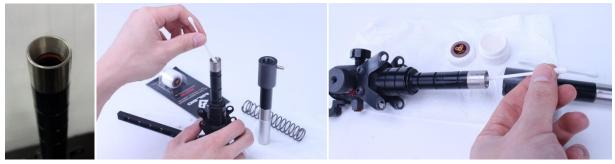
Carefully clean this o-ring with Q-tip and re-oil with SOS lube. This is the most important maintenance step. This o-ring is made from special material for the most critical and demanding seal in the system. Do not use anything other than well mixed SOS lubricant. (Viton® Fluoroelastomer O-Rings Resists chemicals and oil.)
