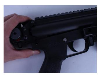
Pivot the lower grip back into place and insert the lower pin.
