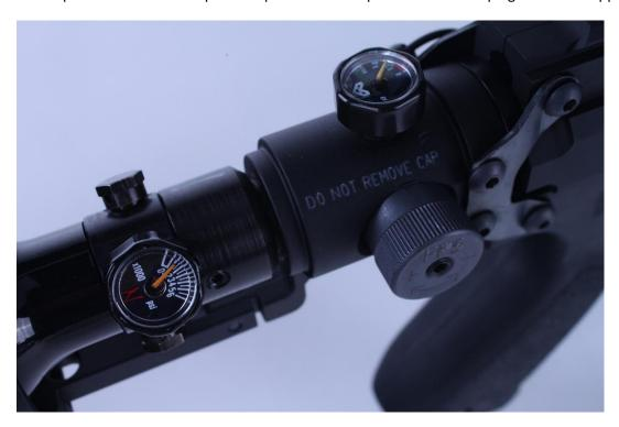
Figure 15 Marker's pressure-gauge indicates the marker's pressure is below green zone. Chances of burping increases.
