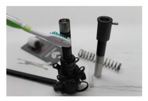
Figure 9 Clean the surface of Gas Chamber and Nozzle interface.
