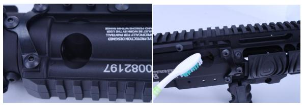
Run a squeegee through the marker barrel with warm soapy water until paint and or damage debris are removed. Use a tooth brush for stubborn paint. Then wipe dry with paper towel and blow dry.
