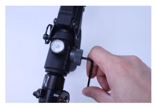
Figure 14 Dial down the fps to your field's limit. Fire twice to allow marker's pressure to stablize.
