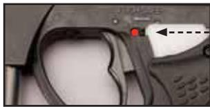
The safety is a small mechanical slide on the left side of the marker above the trigger. When the safety is "off," a red dot is visible on the marker. The trigger can still be pulled if the safety is "on," but the marker will not fire or de-cock.
