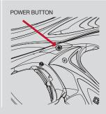
Turn on the marker by holding the power button down for approximately 2 seconds. The marker will turn on with Vision mode activated. The light will blink slowly if there is no paintball in the breech, or rapidly if there is. To de-activate Vision mode, press the power button briefly and it will blink in a double-tap sequence. Press it briefly again to re-activate Vision mode. Press and hold the power button for approximately 2 seconds to turn the Epiphany off.
