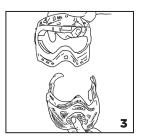
Inspect the mask attachment carefully. Make sure that there are no gaps between the mask and the goggle frame.
