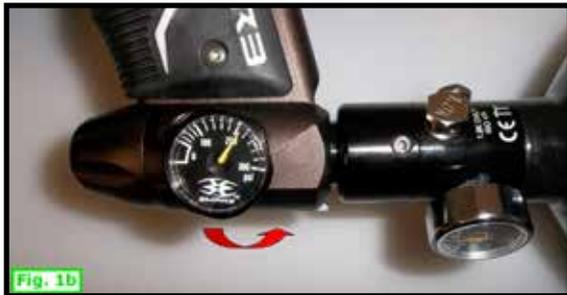
2. Install a compressed air tank, by screwing it in clockwise; making sure it's fully threaded into the ASA.
