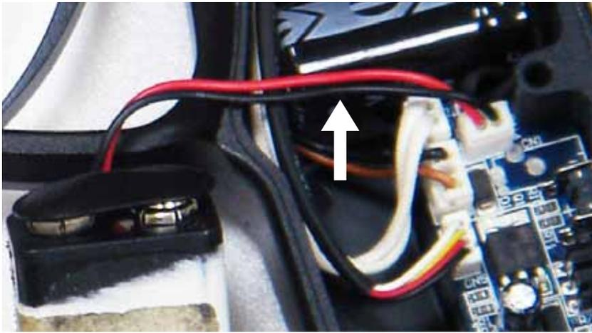
**POSSIBLE CAUSE:** Battery harness is damaged.
