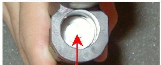
8. Remove cup seal. Use extreme caution not to scratch or damage cup seal. It is recommended to replace the cup seal every time it is removed. Any small scratch or fragment on the cup seal will induce an air leak.
