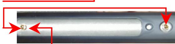
10. Remove air barb from middle of sleeve. Do not loose fiber washer at base of air barb.
