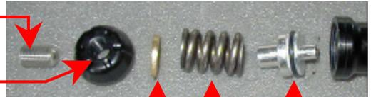
10. Remove Pin Valve Retainer.
