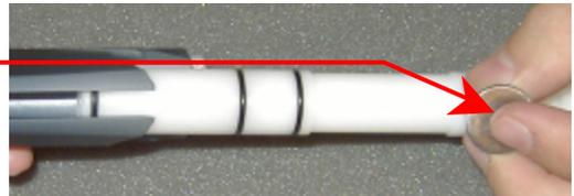
5. Remove rear sleeve cap screw.
