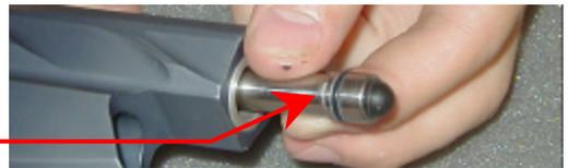
7. Remove poppet from sleeve front. Use a small pair of pliers to grab poppet end. Do not use force on poppet. Poppet will come out with little or no pulling pressure. Use care not to damage poppet lip. Damaging poppet lip will not allow the poppet to seal properly to the cup seal.
