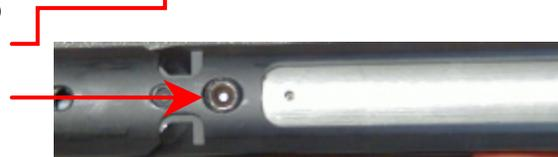
11. Remove sleeve retaining allen.
