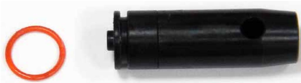
**POSSIBLE CAUSE:** Striker O-Ring is damaged.
