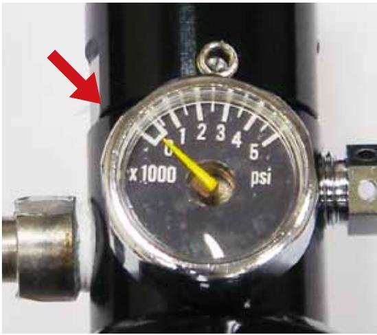
**POSSIBLE CAUSE:** insufficient air supply ( HPA).
