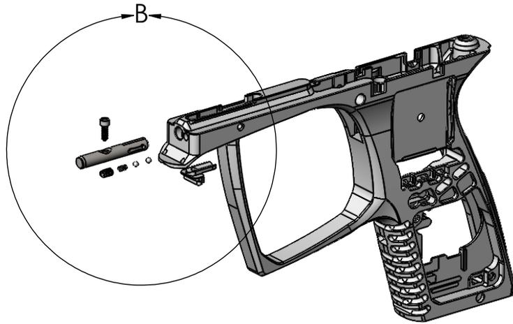
1. INSERT BOTH BAL001 AND SPR007 IN TO SMALL BORE
