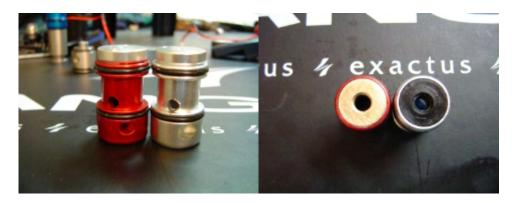
The biggest improvement in the LPR is (again) the gas gallery of the main piston. The piston air channel has been dramatically increased, so you'll need a new piston removal tool. In addition the shims on the LPR piston have also been redesigned to allow more airflow and more wear and tear. However the pressure fluctuation shims still remain the thin paper-like material.
