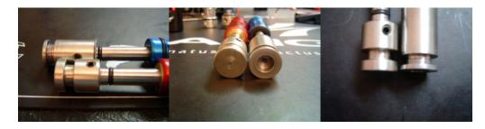
The reason for the redesign is to accommodate the back plate lever. This lever adjusts the ram stroke per say. With the level in the closed position the breech cannot be opened as the bolt is actually pushed forward to sit flush with the rear of the firing chamber. Only when the lever is in the open position can the breech be opened. So the ram has been redesigned to allow the bolt to be moved forward and back in the breech independent of the actual cycling motion.
