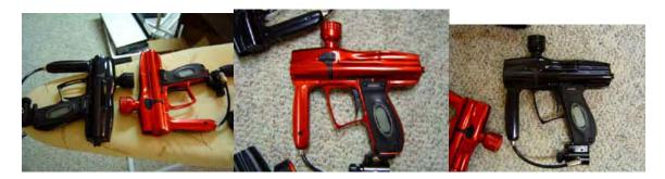
While good anodizing can cover up most milling flaws or tool marks the milling on the G7 is smooth, consistent and clean. You'll notice that they even shaved off some material from the trigger frame and the bottom of the receiver body where the vernier wheels reside.
