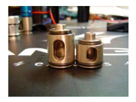
Although it's difficult to see just how different the exhaust valve is from the breech, you'll notice immediately upon removing the component that it is much longer. In addition to being longer the gas galleries have been increased dramatically. The amount of airflow improvement here and the channel to the breech is incredible. More volume, less pressure!
