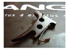
The trigger buffers (on each pivot point) are not installed when the marker is shipped from factory, but they do come in the spares kit that come with each new G7. I actually found that the trigger buffers did not fit when I went to insert the trigger without some effort and once they were in place the free flowing pull of the trigger was much stiffer due to the friction of the buffers. I strongly recommend keeping them removed.
