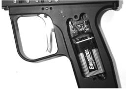
Remove the 2 screws that hold the grip panel in place. Connect the battery to the terminal and place the battery inside the frame carefully being sure that the black and red wires to the terminal are toward the top. Make sure that there are no abrupt kinks and the wires are comfortably placed, do not force them into place. Replace the grip panel and 2 screws.
