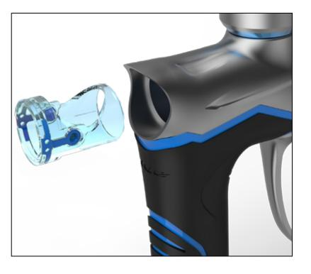
remove the eye pipe/detent system from the front of the marker and unclip the detents for a thorough cleaning. Reinstall the detents, and eye pipe after you have sufficiently cleaned the detents and breech.
