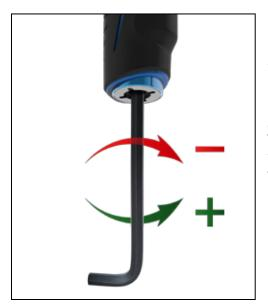
You can adjust your velocity through the Hyper6s Pro™ regulator, located in the fore grip. To adjust the velocity, insert a 3/16" Allen wrench into the bottom of the fore grip. Turning the Allen wrench clockwise, or in, will lower the output pressure, decreasing the velocity. Turning the adjustment screw counterclockwise, or out, will raise the output pressure, increasing the velocity.
