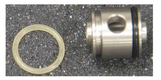
POSSIBLE CAUSE: Front Valve O-Ring (R012) is damaged
