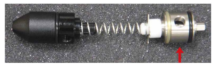
**POSSIBLE CAUSE: Damaged Valve**
